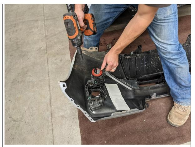
44. Remove fog lights from bumper by removing the 4x Phillips head screws securing them.
