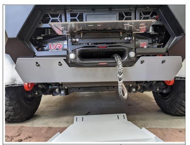
88. Fit bash plate to the front of the bar as shown with 4x M8x30 black button head bolts, black washers and flange nuts. Let the bash plate hang from these fasteners at this stage.
