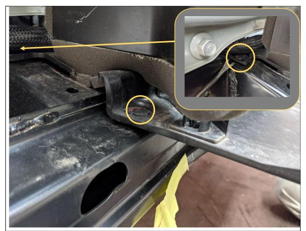
27. Remove lower air guide by removing 4x clips; 2x front (Main Image) and 2x rear (Inset image).
