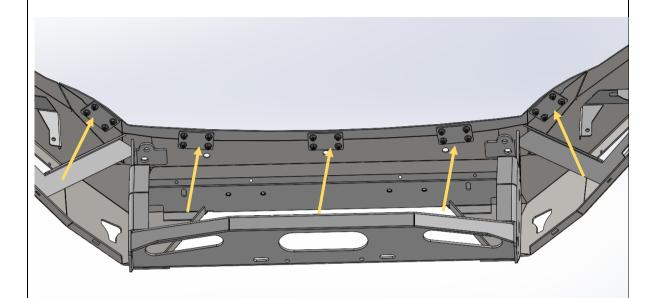
54. Fit the infill panel to the back top edge of the bar, using the supplied M6x16 black button head bolts, flat washers and flange nuts.
