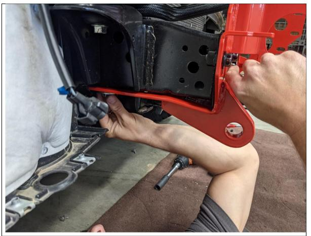
37. On RHS, secure mount to bottom of chassis rail using M12x40 hex bolts, flat washers and M12 nut plates inserted through front of chassis rail.
