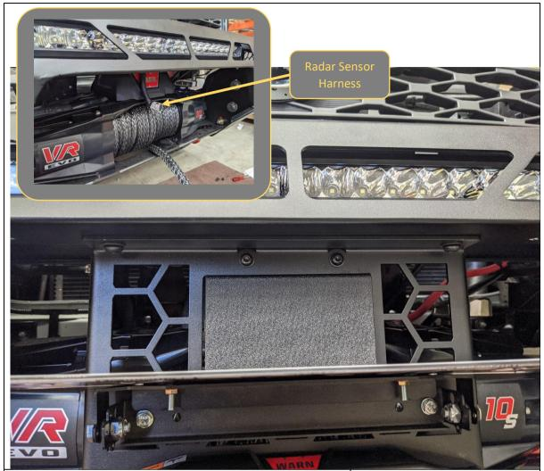
82. Pre-Position radar sensor harness to front of opening.
