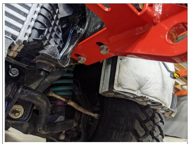
36. On LHS secure bottom of mount to nuts in chassis rail using factory 17mm hex bolts removed from tie down point.
