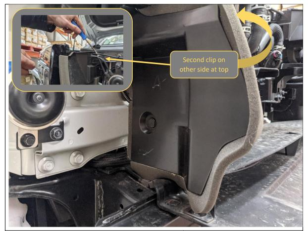
22. Remove and retain upper air guides. These are secured with 2x clips. These will be modified and refitted.
