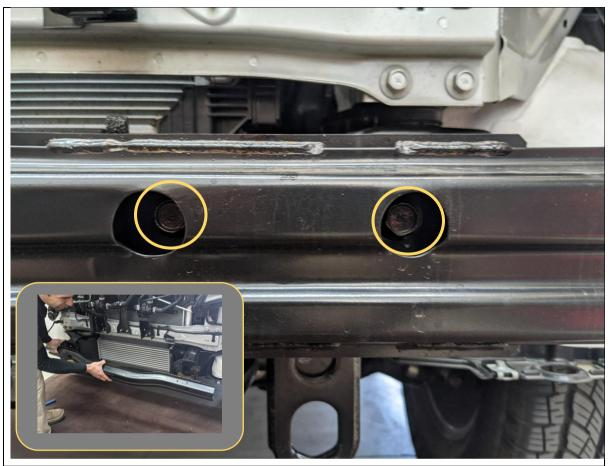
30. Remove all 4x bolts securing crash beam, then remove the impact beam.
