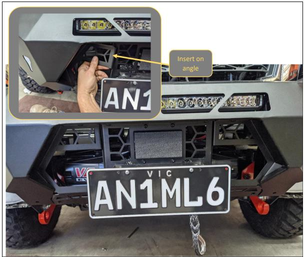
85. Fit Mesh Infill Panels. Use 1x M8x16 black button head bolt and M8 black washer into the captive thread in the bull bar.
